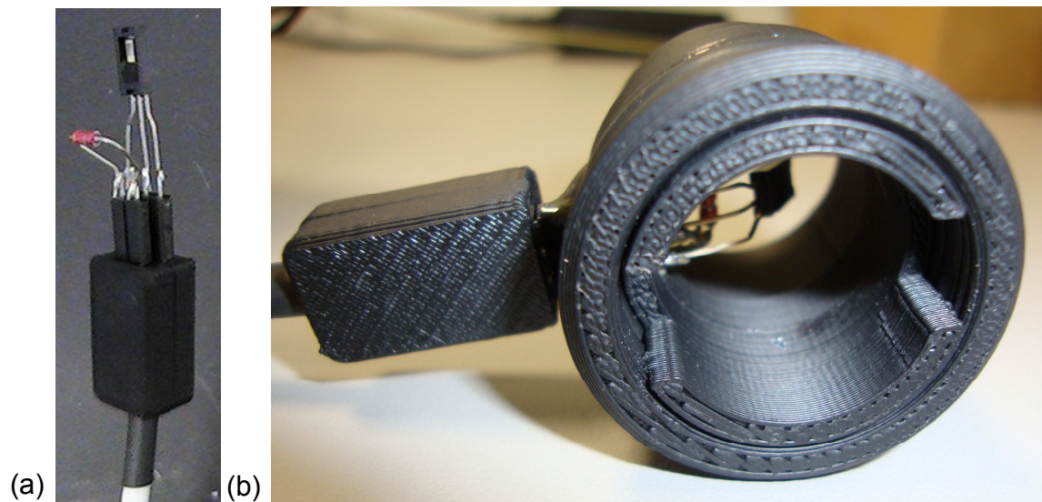
Figure 3.2 External humidity-temperature sensor: (a) Combining the HIH-4000 humidity sensor (black) and NTC 198-927 thermistor (red); (b) Attachment of the sensors within the ABSplus 3D cap.
