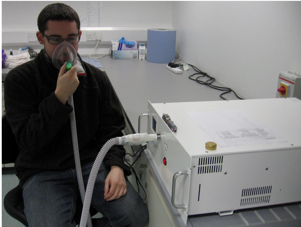
Figure 2.2 Breath ammonia measurement using photoacoustic spectroscopy. The typical procedure for volunteer breath collection using PALS.
