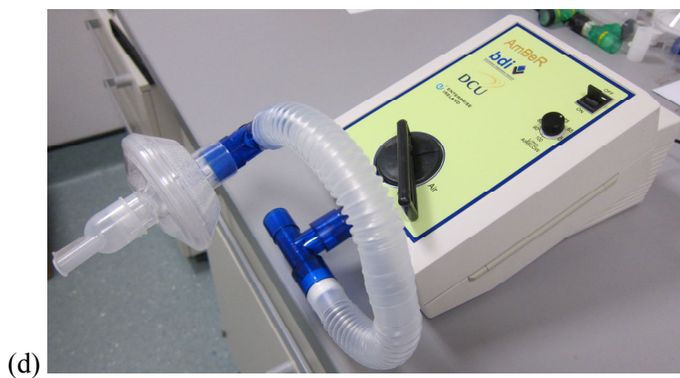
Figure 5.11 Final AmBeR design prototype. (a) Schematic of the device and air flow direction, (b) photograph showing internal assembly, (c) photograph of disposable sampling chamber portion, and (d) photograph of final assembled prototype.
