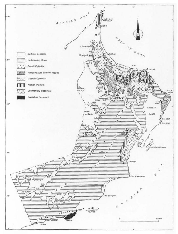
Fig. 1- Geological sketch map of the Sultanate of Oman (from Le Metour et al., 1995).
