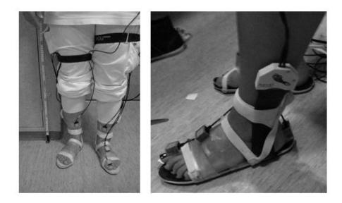
Figure 7: Sensor placement for the ambulatory gait assessment system. On the tested ankle (left side) sensors are placed at the dorsal aspect of the proximal phalanx of the first toe, between the bases of the first and the second metatarsals, the great tuberosity of the calcaneus.
