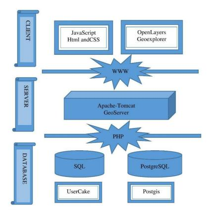
Figure 3 Architecture of the Web-GIS platform
