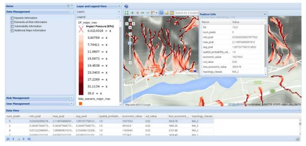
Figure 4.13. Visualization of the calculated loss scenario, illustrating the affected buildings with economic losses for the debris flow major event (maximum intensity in KPa).
