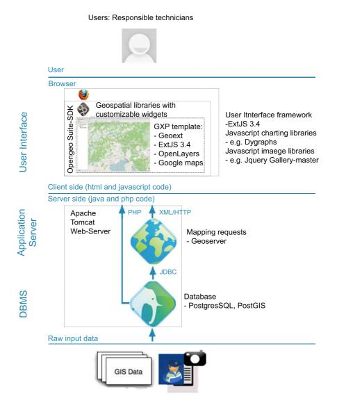
Figure 3: System architecture of the web-GIS platform based on Opengeo Suite. \*Volunteer icon (Civil Protection of FVG region, Italy)
