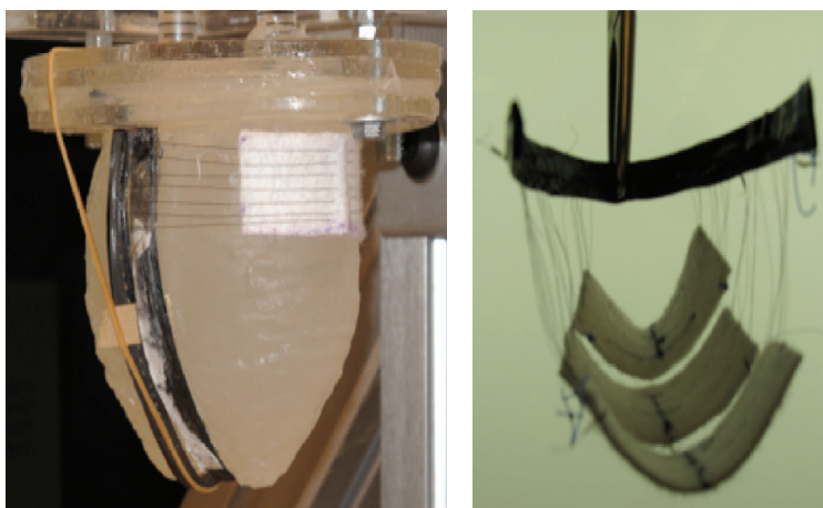
FIGURE 5: Wires around the ventricle with a slice of PTFE between the wall and the wires.
