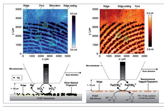
Top: Constant height SECM images of a fingerprint developed by silver staining (left) or benzoquinone tagging (right). Bottom: Schematic representation of the detection principle of silver nanoparticles containing fingerprints (left) and benzoquinone-tagged fingerprints (right).
