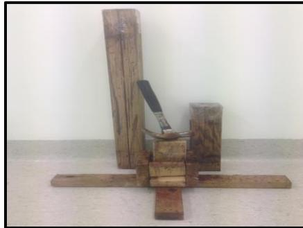
Figure 13 Wooden apparatus and hammer used to create impact patterns (Evans, 2015)
