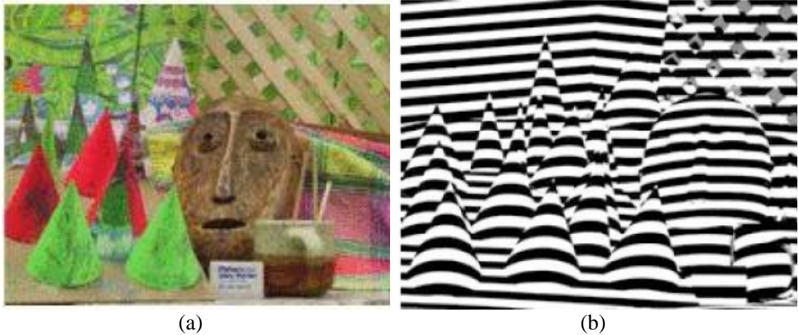
Figure 6. Example image of structured light reflected off surface (a) original scene, (b) thresholded gray-code image (19).
