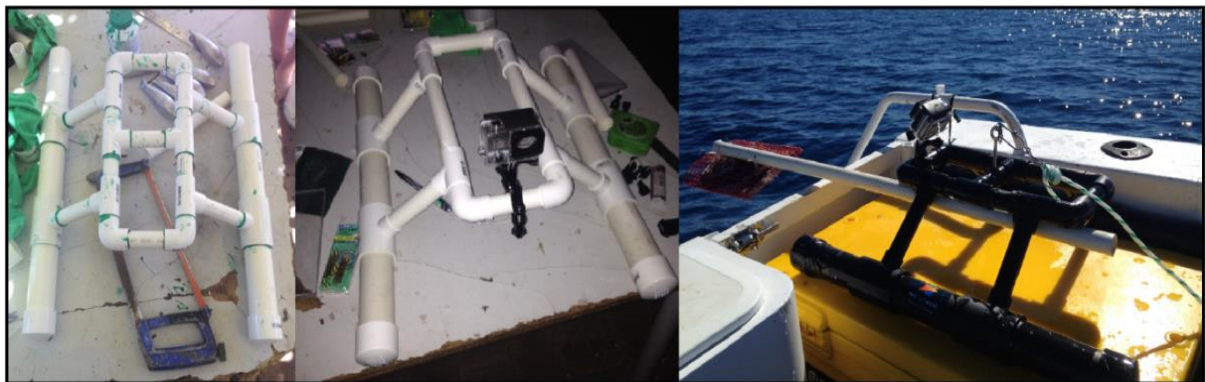
Fig. 15. Construction of the custom made BRUV. From right to left: Cementing pipe fixtures with weights already inside the legs (skids), the finished BRUV frame trialling with camera position, and final product about to be deployed on the artificial reef.
