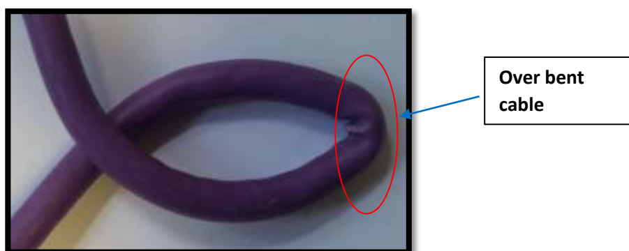
Figure 23: Example of over bent cable
