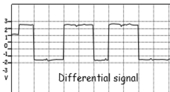
Figure 4: Properly terminated signal [13]
