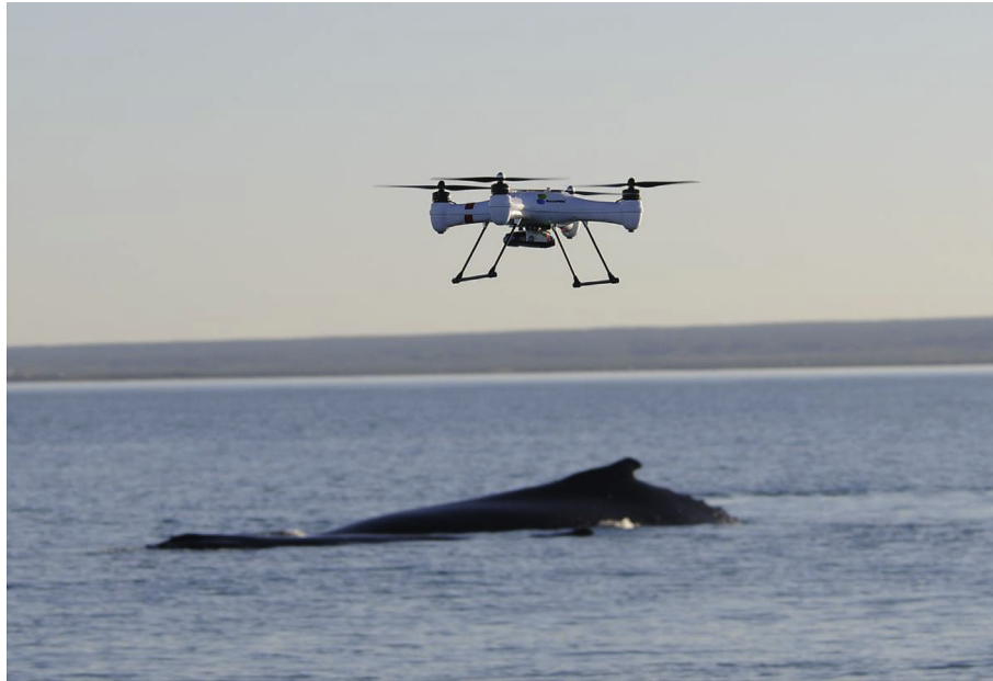
Figure 1. Quadcopter unmanned aerial systems (UAS) hovering in the foreground with a humpback whale in the background. Although it appears large, the copter is 500 mm in diameter and 230 mm in height, with landing gear. These platforms, multirotors and fixed-wings are being used to collect data of several types (e.g. photogrammetry, exhalent samples, thermal imagery). Given the rapid acceleration in the UAS technology, we expect the use of these systems to increase for behavioural as well as other research applications.
