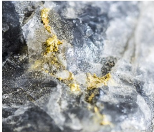
Fig. 1 Elemental gold embedded within a quartz matrix from a West Australian mine
