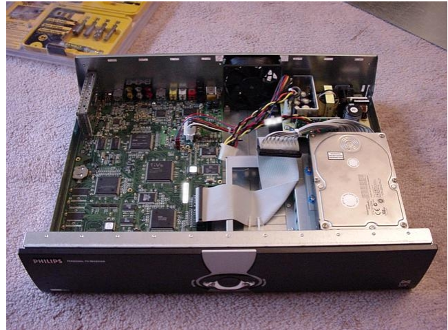
Figure 2. TiVo Series 1 as used in Australia by the OzTivo community. The case is shown open, as required to access the hard disk in order to set up unit for Australian use.
