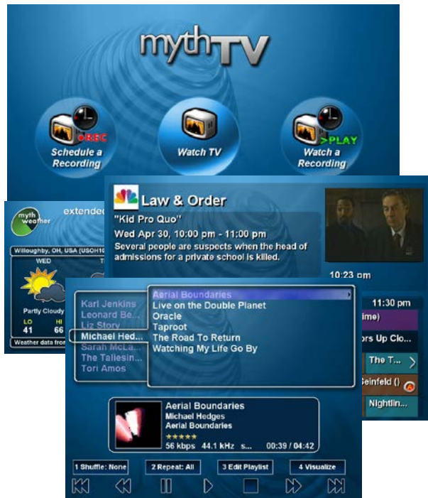
Figure 3 Screen shots of MythTV, showing various available functions: menu and PVR function with EPG scheduling weather, music player, and photo viewer.
