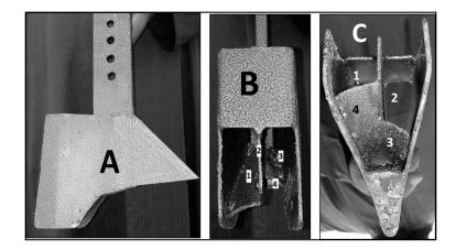
**Figure 4.** Side (**A**), back (**B**); and bottom (**C**) view of a newly developed furrow opener with the capacity to separate seed and fertilizer; B1/C1 = seed delivery channel, B2 = seed and fertilizer separator, B3/C2 = fertilizer delivery channel, B4/C3 = soil scraper to ensure about 20 mm soil layer between seed and fertilizers.
