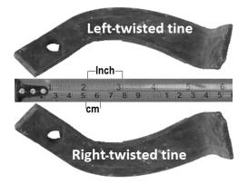
Figure 5. Photograph of right- and left-twisted tines.
