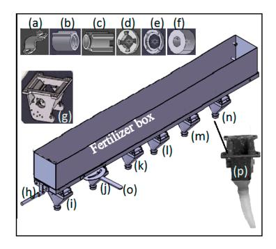
**Figure 3.** Fertilizer box with metering mechanism; (**a**) nose clump; (**b**) bush; (**c**) fluted roller type fertilizer meter; (**d**) roller regulating bush; (**e**) bush cover; (**f**) bush clump; (**g**) fertilizer meter housing; (**h**) fertilizer meter regulating shaft; (**i**–**n**) fertilizer dropping funnel (six rows); (**o**) fertilizer rate control/adjustment lever; (**p**) a complete seed metering mechanism for one row having (**a**–**g**) parts.
