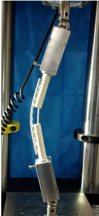
Figure 6 – An LCPR construct in axial load to failure. Each construct was mounted vertically and axially loaded through 25mm ball bearings at either end. All constructs failed by plastic deformation of the plate.
