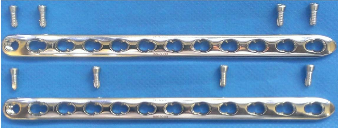
Figure 2 - Two screw configurations were used, the first with screws at 1 and 2, modelling the long (8 holes) working length, and the second, with screws at 1 and 4 modelling the short (4 holes) working length.
