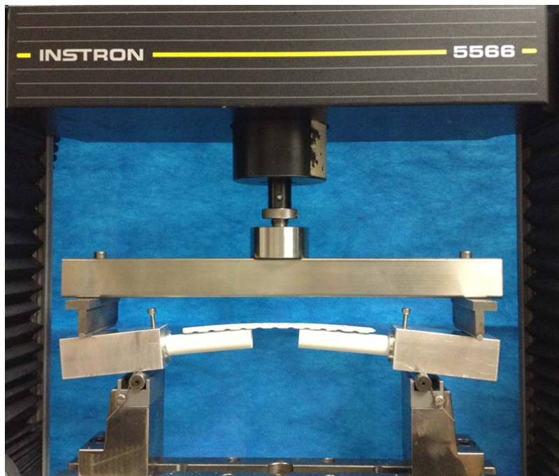
Figure 5 – An LCPMono construct tested in non-destructive mediolateral bending. Each construct was manually centred using a 300mm gap between the two support rollers and a 220mm gap between the load rollers. The materials testing machine applied a constant bending moment along the plate.
