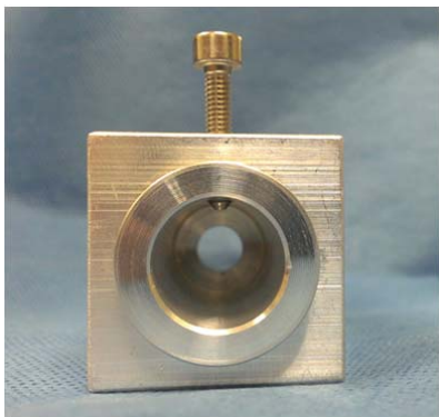
Figure 1 – Two custom designed loading jigs were made with an 8mm central hole to avoid any impingement on intramedullary pins protruding from the constructs during testing.
