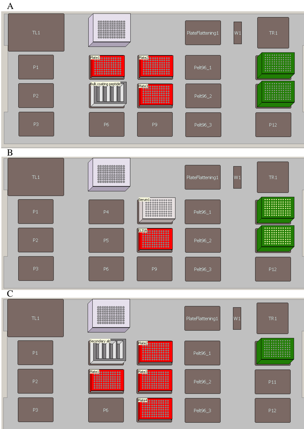
Supplementary Figure S-3. ELISA protocol steps robot layout on BioMek. Coating plates (A), sample addition (B) and secondary antibody addition (C) using appropriate reagent storage, pipette tips (dark green) and ELISA plates (dark red).
