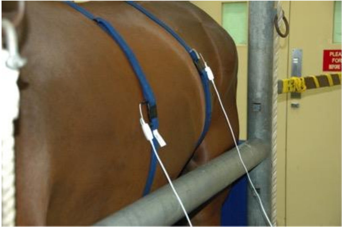
Figure 4: Thoracic and abdominal respiratory inductance plethysmography (RIP) bands were placed between the 9 th and 11 th intercostal spaces and behind the last rib respectively
