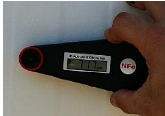
Figure 3.21a: Coating thickness measurement
