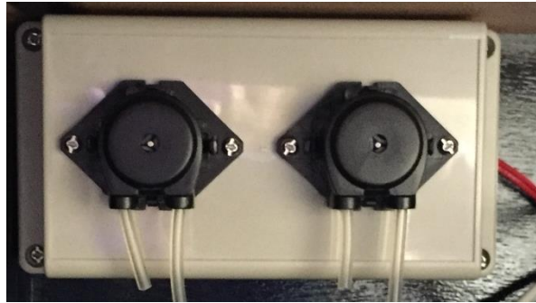
Figure 6-6 – pH Dosage Pump (left), Fresh Water Dosage Pump (right).
