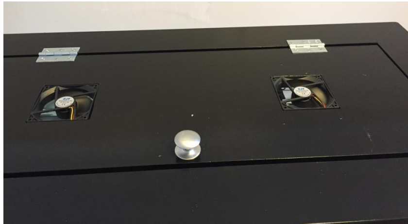
Figure 7-4 – Controlled Exhaust Fans at the Top of Lighting Hood.
