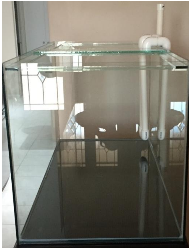
Figure B14 – Completed Siphon Drain Setup for the Project.
