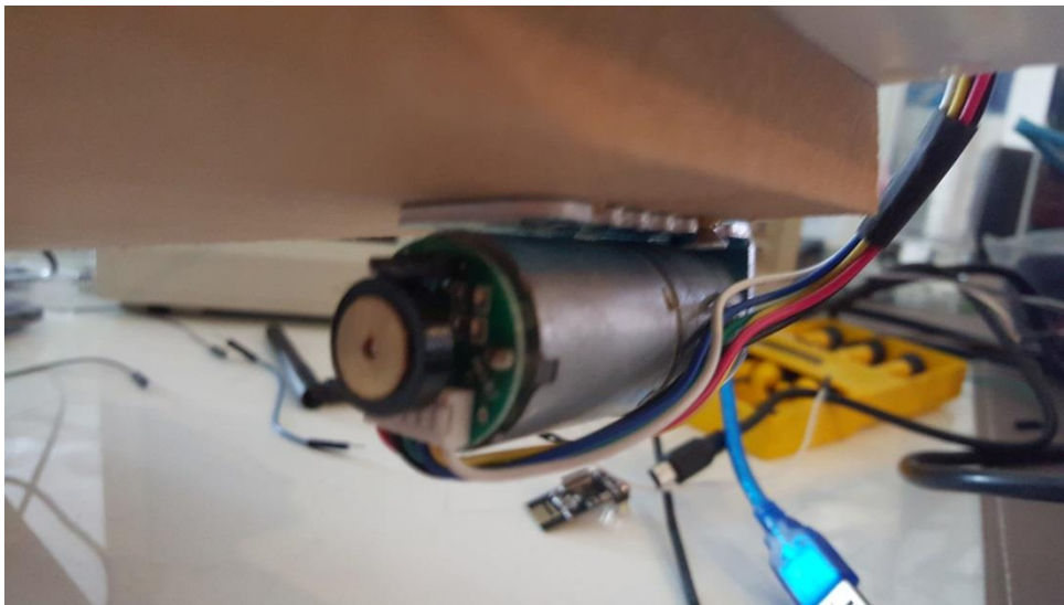
Figure 13: Motor and Encoder on motor bracket [42]
