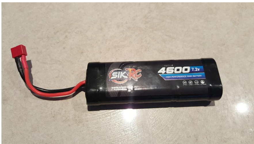
Figure 16: SIK RC 7.2V 4600mAh Ni_MH battery [42]
