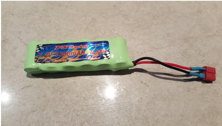
Figure 15: FS Racing 7.2V 1300mAh Ni-MH battery [42]
