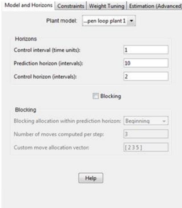
Figure 39: MPC Controller Parameters in the MPC Toolbox in Simulink.
