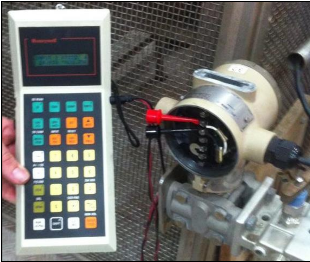
Figure 8: Ball Mill Level Calibration
