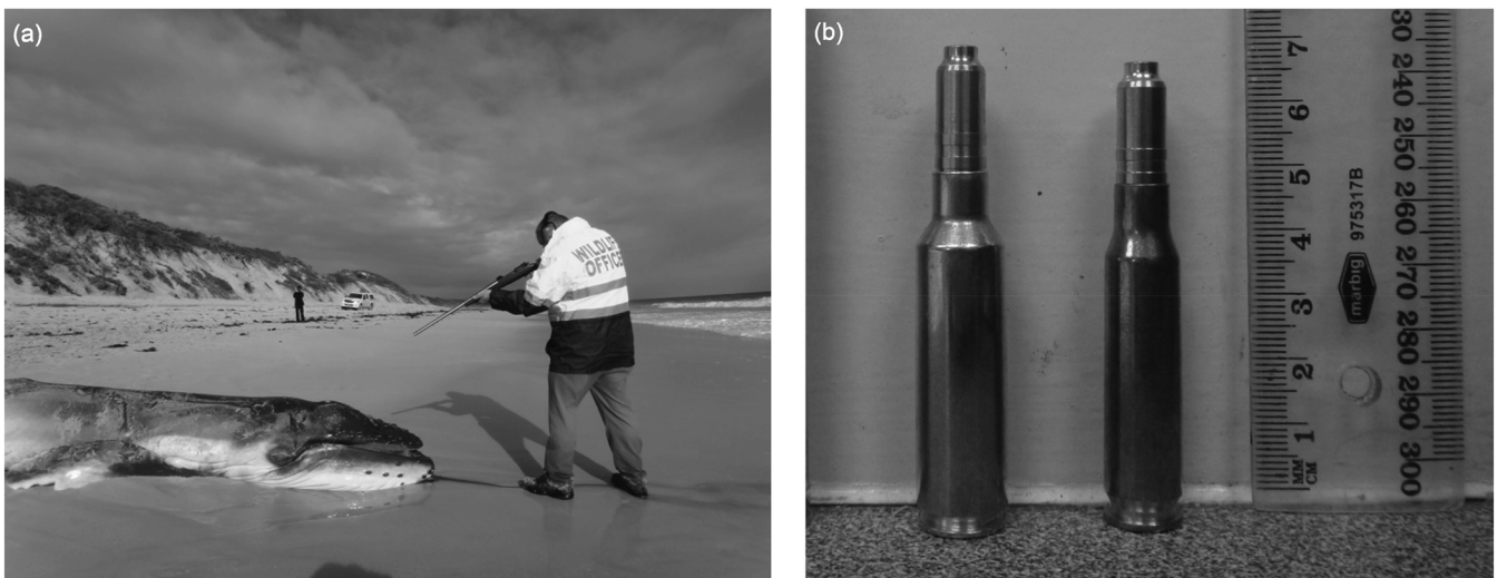
Fig. 1. Standardised shooting methodology used in this study. (a) Standardised shooting technique for post-mortem ballistic testing on a neonate humpback whale ( Megaptera novaeangliae ) in ventral recumbency. (b) The non-traditional design of the .30 calibre blunt solid copper-alloy non-deforming Woodleigh hydrostatic projectiles used for standardised shooting. The shell casings are .300 Winchester Short Magnum (left) and .308 Winchester (right).
