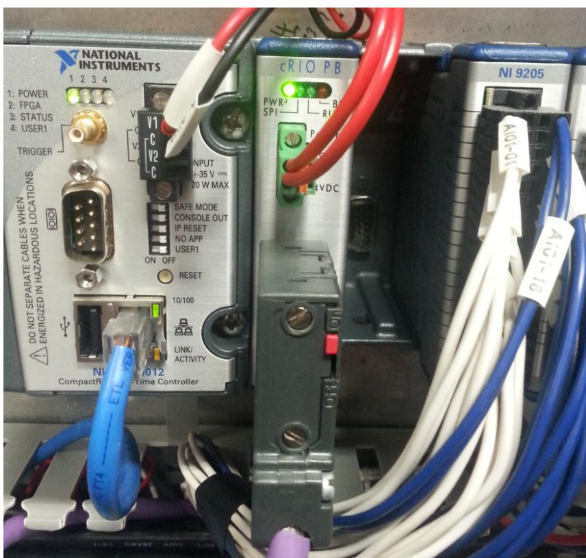
Figure 7 - cRIO PB Module installed in chassis
