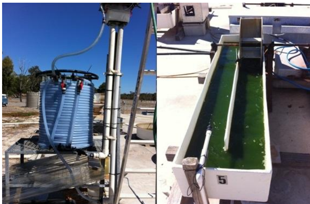
Figure 4. 40 L Biocoil-type tubular photobioreactor (Left) and 200L paddle-wheel driven raceway pond (Right) used in this study.
