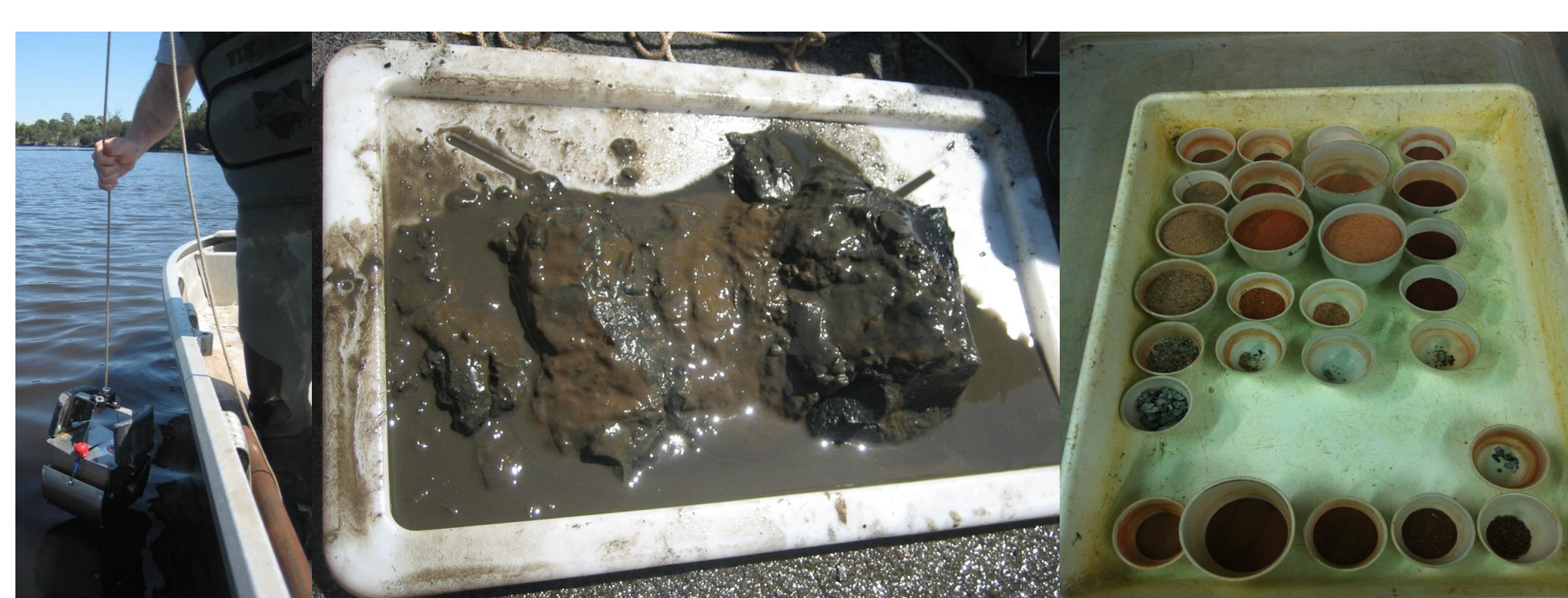
Fig. 3: (a) Sampling with an Ekman grab, (b) typical sediment from deep waters and (c) sifted inorganic fractions.
