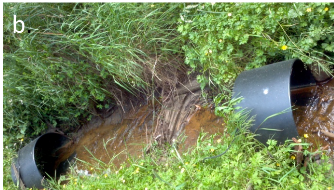
Fig. 2. Showing the three Units placed in the field. a) Unit 1, the ANT612 flat panel antenna (arrow) in the creek at Site A, and b) Units 2 and 3 (C600 swim-through tunnels) placed in line at Site G.
