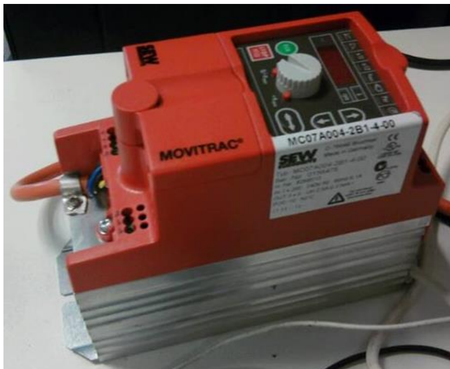
Figure 9 - Isometric view of the unit which is rated for 0.37kW AC machines
