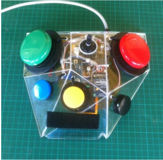
Figure 23, Different Joystick and Velcro Added
