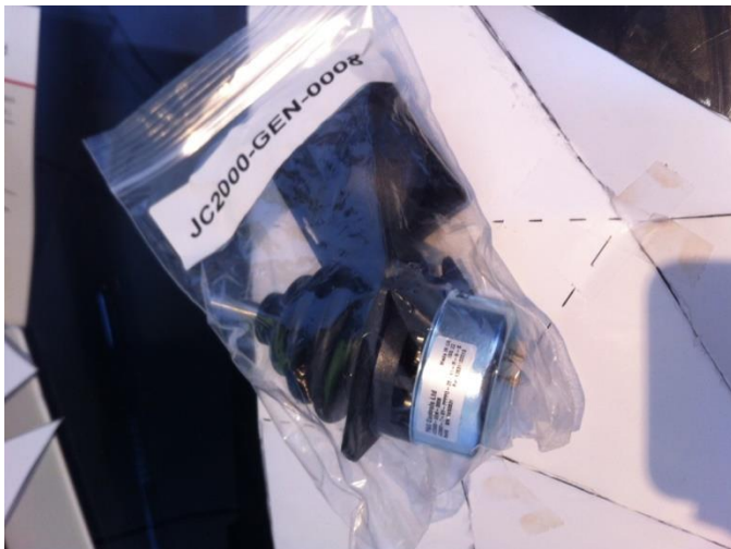
Figure 31, Right Joystick - Penny and Giles, JC2000
