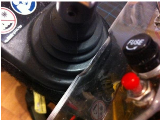
Figure 28, Back of Left Controller Locked onto the Chair's Joystick Base
