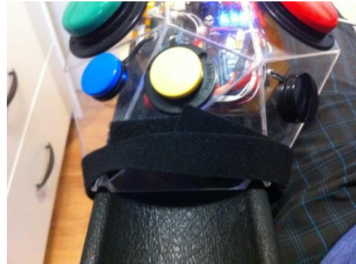
Figure 27, Left Controller Locked in Arm Rest by Grooves
