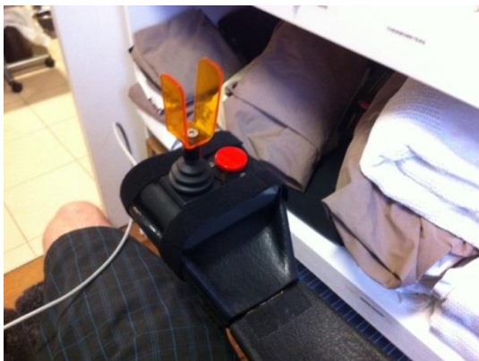
Figure 34, Right Controller fitted to Arm Rest
