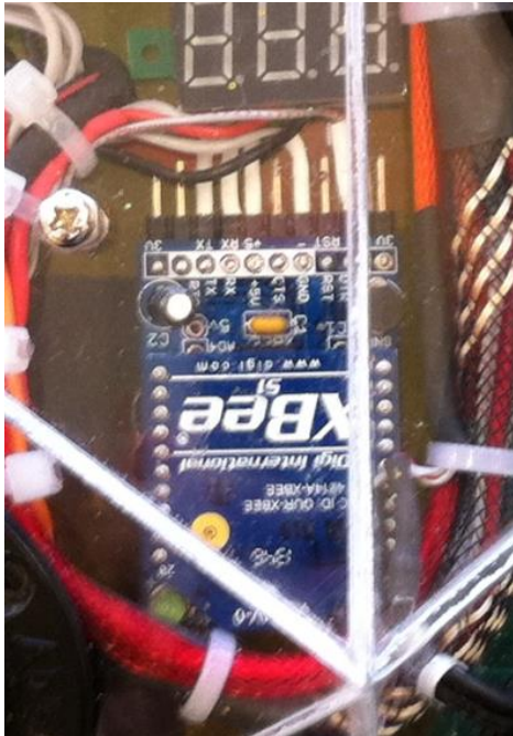
Figure 43, Xbee Adapter Soldered onto Headers
