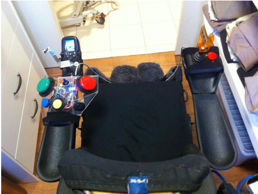
Figure 5, Left and Right Controller Fitted in the Chair with Velcro
