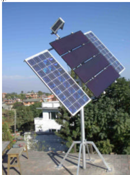
Figure 7. Locally designed and made solar tracker
