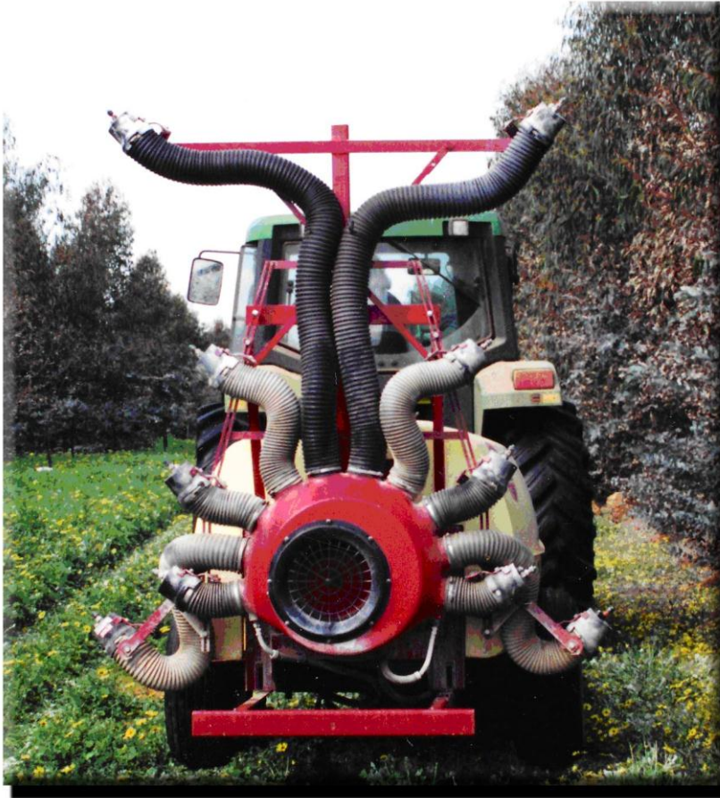
Figure 8.4 The spraying rig used to deliver the fungicides and insecticide to the treated Eucalyptus globulus trees. (Photo by H. Neumeister-Kemp)
