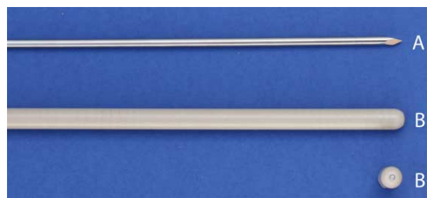
Figure 1 Intramedullary implant types: (A) 2.4 mm Steinmann pin; (B) 6 mm poly-ether-ether-ketone rod with a (B 1 ) modified tip photographed end-on.
