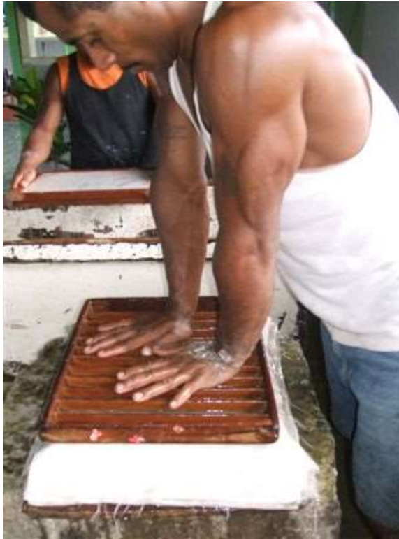
Figure 5.2.2g. They transferred from the mould to the flat couching surface by pushing and rocking the frame until the layer of pulp is transferred.
