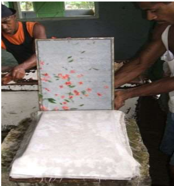
Figure 5.2.2g. They transferred from the mould to the flat couching surface by pushing and rocking the frame until the layer of pulp is transferred.
