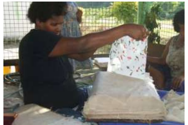
Figure 5.2.2i. Ladies then peeled off each sheet pasted onto a tin drying operation.
