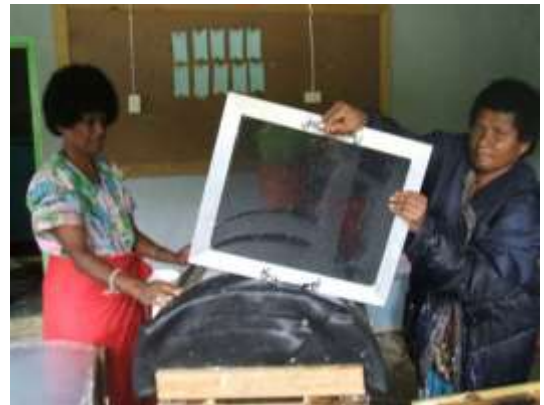
Figure 5.3.2.1mn. Then exit without drips on the delicate paper that would destroy a now valuable sheet of damp paper.
