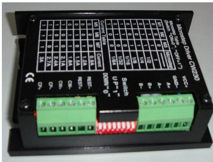
Figure35: CW230 2-Phase Micro stepping motor driver
