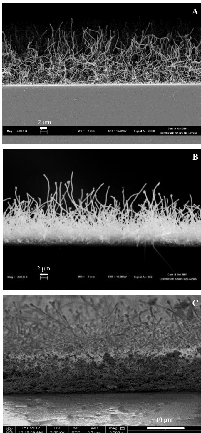
Figure 6.4: Cross-sectional images for SiNWs synthesized using Au catalyst layer thicknesses of (A) 20nm, (B) 60nm and (C) 100nm.
