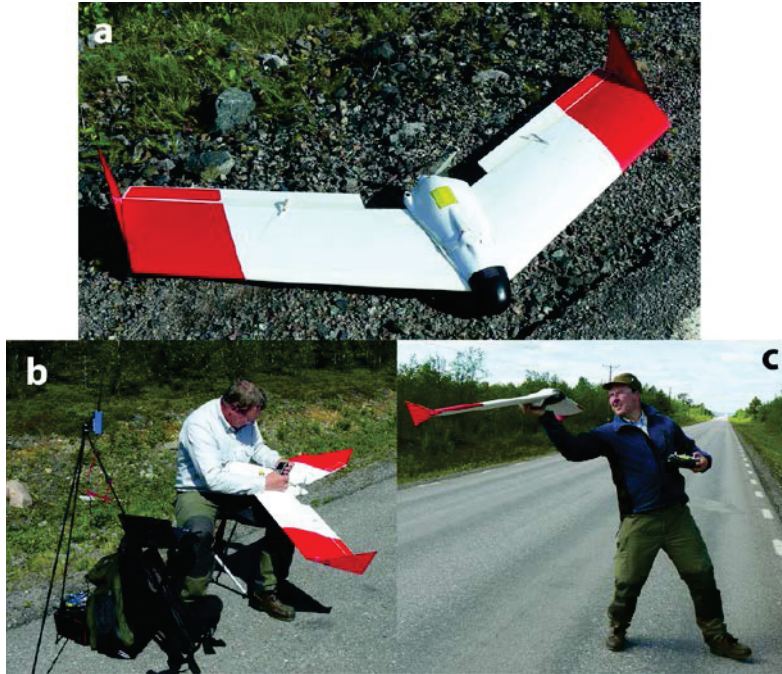
Figure 5. UAS by SmartPlanes Sweden AB; a) SmartOne aircraft, b) control station, c) ready for take-off.
