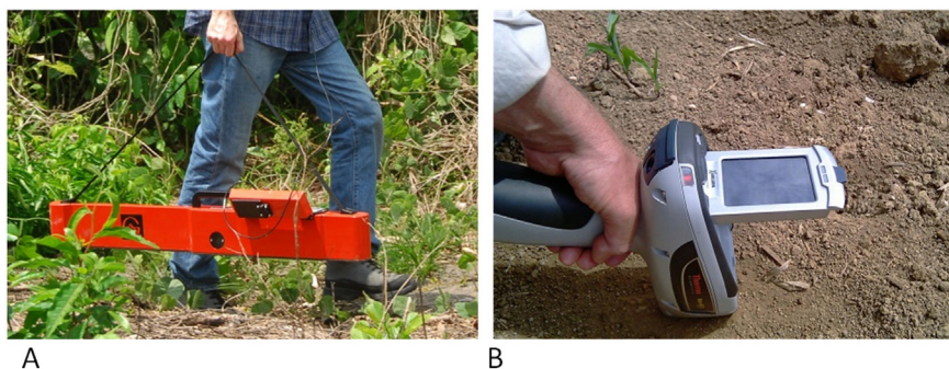
Fig. 3. Proximal soil sensors used: A) EM38-MK2 (Geonics Ltd., Mississauga, ON, Canada) for measuring soil electrical conductivity and magnetic susceptibility (photo: Christian Isendahl); B) Niton XL3t GOLDD+ (Thermo Scientific, Billerica, MA, USA), a portable x-ray fluorescence (PXRF) analyser for detection of the total concentrations of many elements (photo: Mats Söderström).
