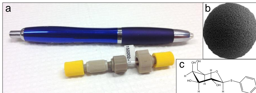
Figure 14. The miniaturized affinity columns were based on Poros ® chromatography material (b), modified with a galactose terminated ligand (c), and packed into conventional peek tubing (a).
