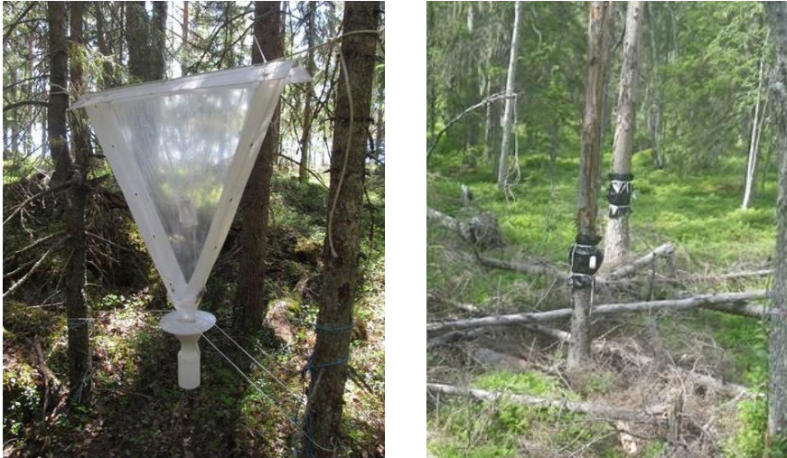
Figure 2: Left hand picture: flight intercept traps used for collecting beetles in Papers I & II, and flat bugs in Paper IV (Swedish part). Right hand picture: eclector traps used for collecting beetles in Paper III. Photo: R. Hägglund
