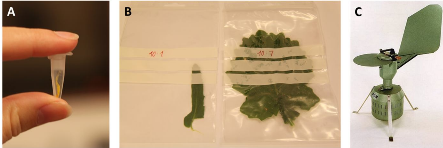
Figure 11. S.sclerotiorum DNA was monitored in three different sample types: (A) petals, (B) leaves from different leaf levels and (C) air samples collected using a Burkard 7 day recording volumetric spore trap. The photo of the spore trap is published with kind permission from Burkard Manufacturing Co. Ltd.
