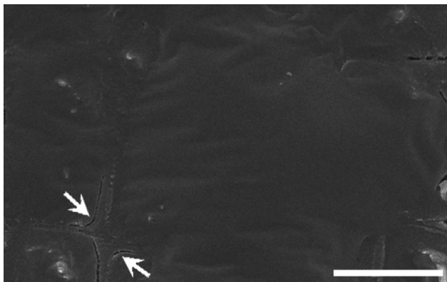
Figure 4 SEM micrograph of wood treated with ELO. TS section of LW tracheids from EA treatment with the cell wall layers and ML regions almost erased; cracks have been induced (arrows) during sectioning. Scale bar, 20 \mu\text{m} .
