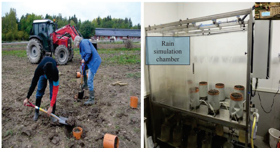
Figure 7. Sampling of the soil monolith (left) and the rain simulation chamber (right) used to investigate nutrient leaching from those soil columns (photo: Nargish Parvin).
