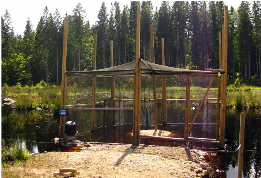
Figure 1. A duck trap was built 2011 to capture wild and farmed ducks for ringing, bill measurements, DNA sampling, and fitting with GPS-loggers. The 4x4x2 meter trap with three funnel entrances is located in a small wetland in northern Scania, southern Sweden (WGS84, 56°26'24.2''N, 13°59'32.5''E). The trap was baited with barley and enclosed with electric wires. Photo: Pär Söderquist.
