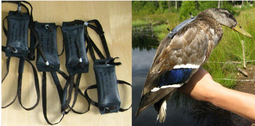
Figure 3. Captured mallards were fitted with a CatTrack GPS-logger (Catnip Technologies Ltd.). The logger was put in a shrinking tube for waterproofing, with a maximum size of 95x30x15 millimeters and a weight of 25 grams, including the Teflon harness. An address was written on the shrinking tube and on paper inside the shrinking tube as information about where to send recovered loggers. Photo: Pär Söderquist.
