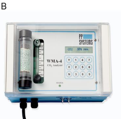
Figure 7. Labelling experiment set up. Two month old wild type (line T89) hybrid aspen trees were placed in a transparent chamber and labelled with ^{13}\text{CO}_2 under controlled environment. The temperature and humidity were kept constant using an air conditioner unit (A). \text{CO}_2 level was monitored by a \text{CO}_2 detector (PP SYSTEMS) (B). \text{CO}_2 injection was performed using a 1 ml syringe (Hamilton) (C).
