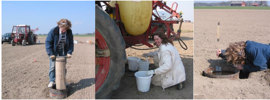
Figure 7. Water infiltrability measurements at Lanna. Left: Insertion of steel cylinders. Centre: Filling of buckets from a water tank. Right: Measurement of water head. Photos: Maria Stenberg.
