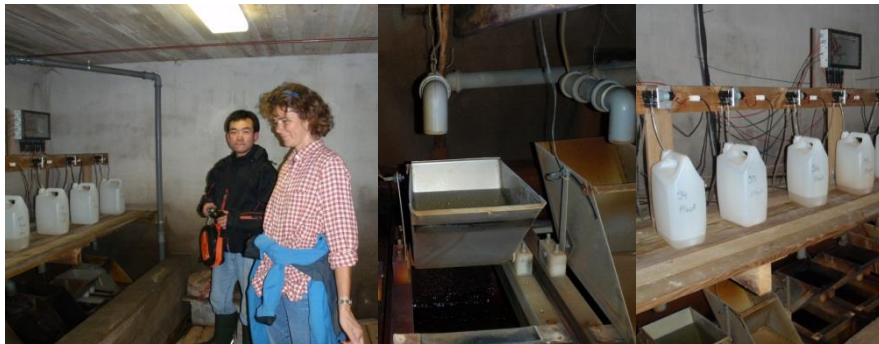
Figure 5. Measuring station for drainage water from the experimental field at Mellby in Halland, with tipping buckets for measurement of draining volumes (middle) and pumps and plastic flasks for collection of flow-proportional water samples (right). Photo: Åsa Myrbeck.
