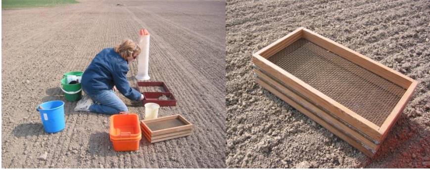
Figure 9. Left: Characterisation of the seedbed. Right: Sieve used for quantification of different aggregate fractions within the seedbed. Photos: Maria Stenberg.
