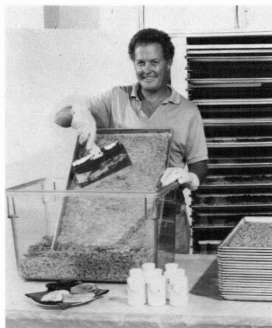
Peter Allen of Papaya Products Hawaii uses geothermal brine to provide heat to produce green papaya powder.
