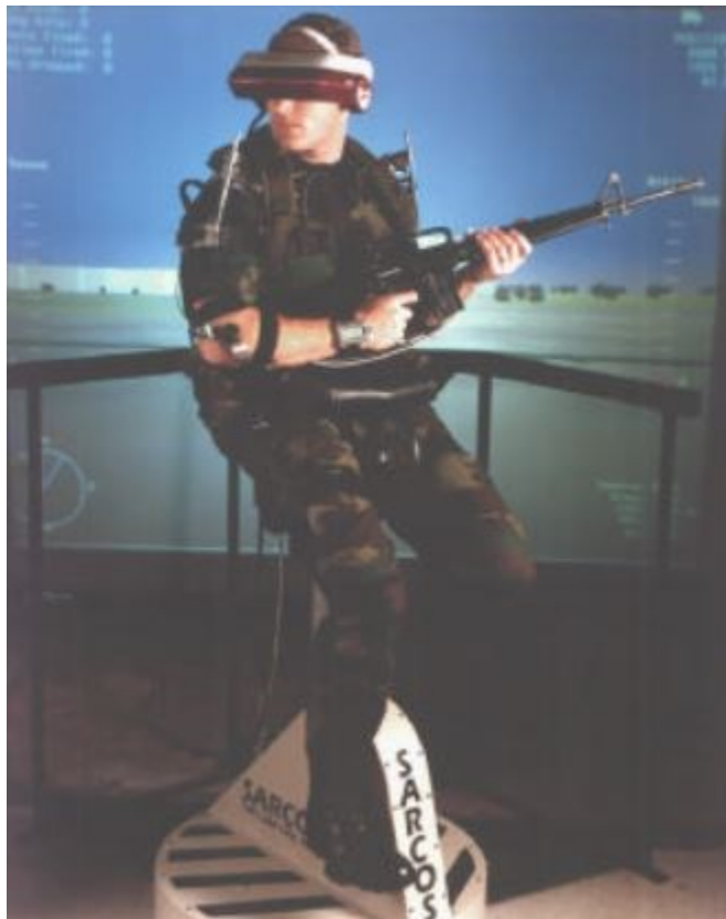
Figure 2-3. Sarcos Uniport locomotion device [80]
