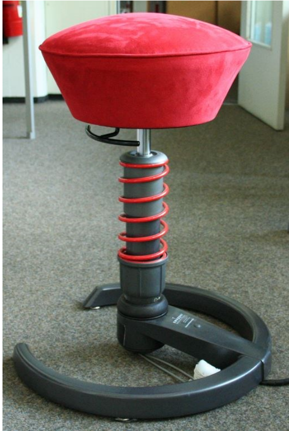
Figure 2-5 The ChairIO is a chair based interface to control navigation in 3D environments or to control cursor movement on the desktop [4]
