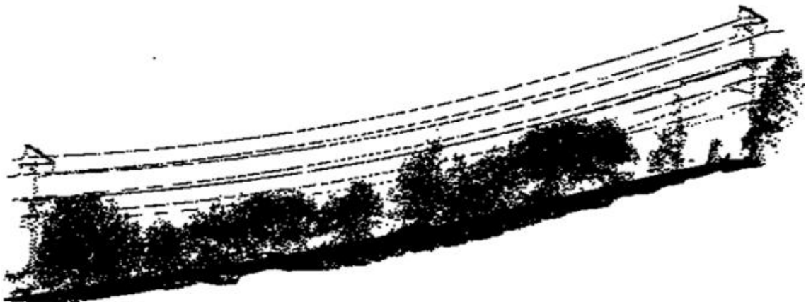
Figure 2.3: Vegetation encroachment to PL components in the PL voltage of 69 kV: points representing PLs and vegetation are mixed, so that it is very hard to discern PL points from vegetation points.
