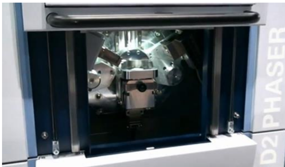
Fig. 2.7: Geometric arrangement of X-ray diffractometer (adapted from reference 57).
