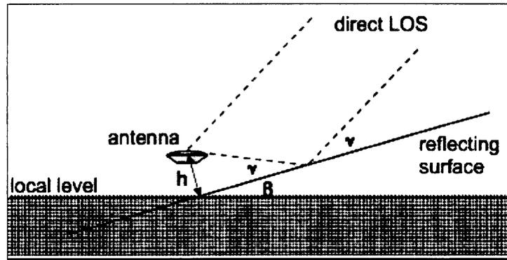
**Figure 4.1: Simplified reflector geometry.** The antenna is at a distance  $h$ , normal to the surface. The satellite line of sight is incident at angle,  $\gamma$ , to the surface. Source: (Axelrad *et al.*, 2005)
