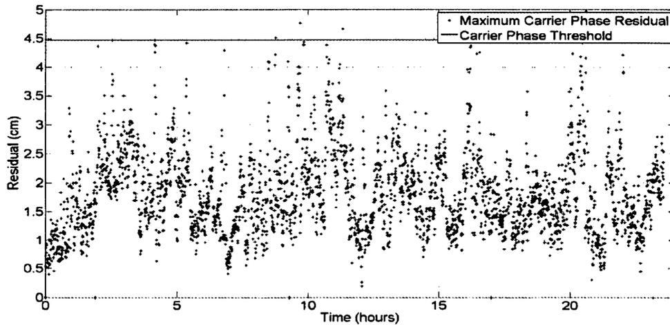
**Figure 3.20: Fixed threshold residual rejection**
