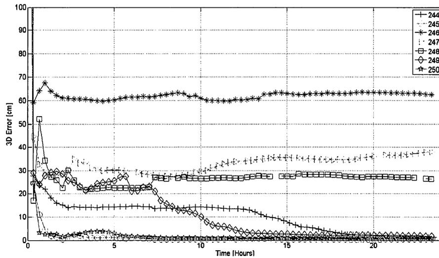
**Figure 3.3: Site KIRU showing poor convergence static mode**
