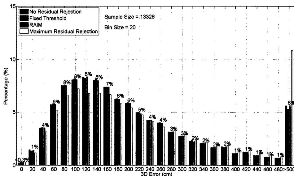
**Figure 3.22: Distribution of the 3D position error used to initialize the PPP filter**
