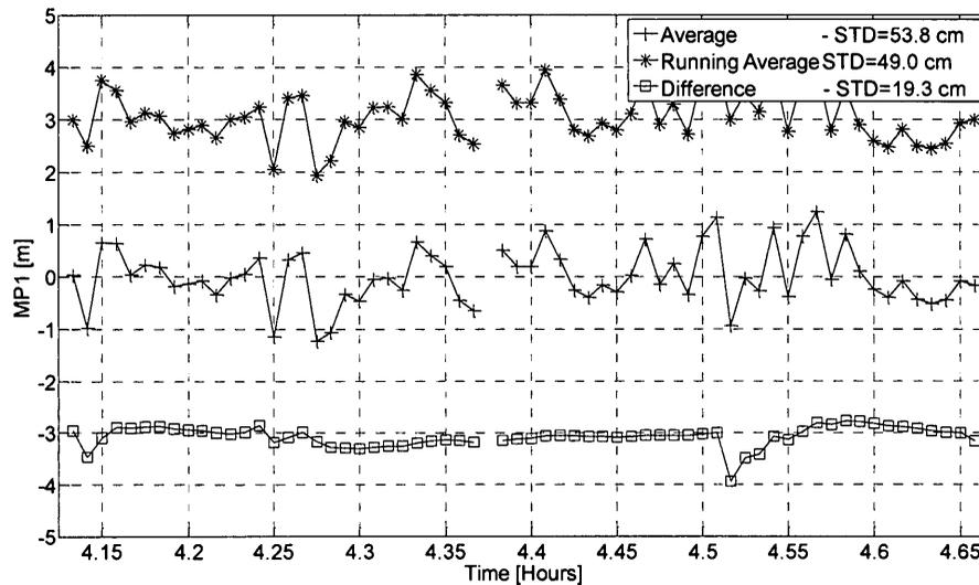
**Figure 4.13: Pseudorange multipath for PRN 03 at KIRU, for DOY 249 using running average, in elevation range of 10-30°**
