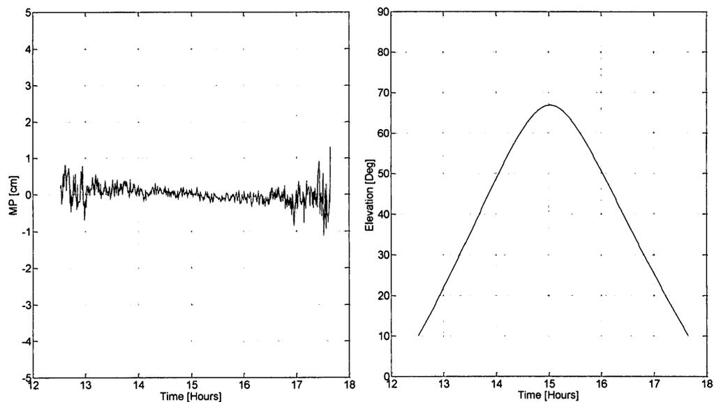
**Figure 4.7: Ionospheric free pseudorange multipath observable (left) and elevation angle (right) for PRN 03 at Algonquin (ALGO) on DOY 249**
