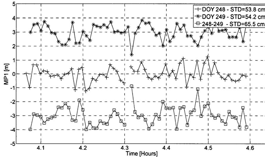
**Figure 4.11: Pseudorange multipath for PRN 15 at KIRU, for DOY 248 and 249 in elevation range of 10-30°**
