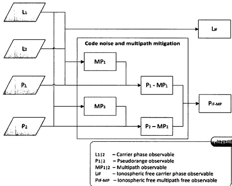
**Figure 4.14: Measurement processing flow augmented by multipath mitigation modules**
